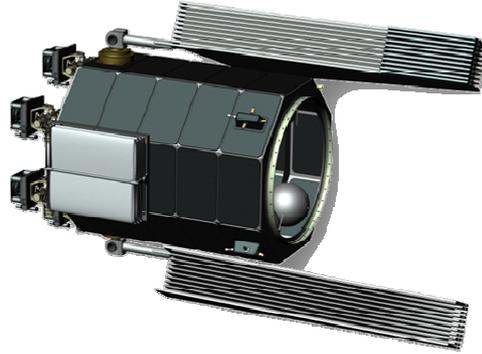
**Fig. 4: Notional 30kW SEP Module Design**
